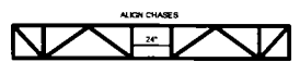
FOR SPANS FROM 12'-0" TO 22'-0" (1) ROW IS RECOMMENDED AT THE APPROXIMATE MID SPAN. FOR SPANS FROM 22'-0" TO 30'-0" (2) ROWS ARE RECOMMENDED AT THE APPROXIMATE THIRDS POINTS OF THE SPAN.
